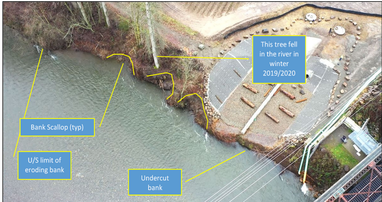
Figure 2.4: December 2019 UAV image annotated with erosional features.
